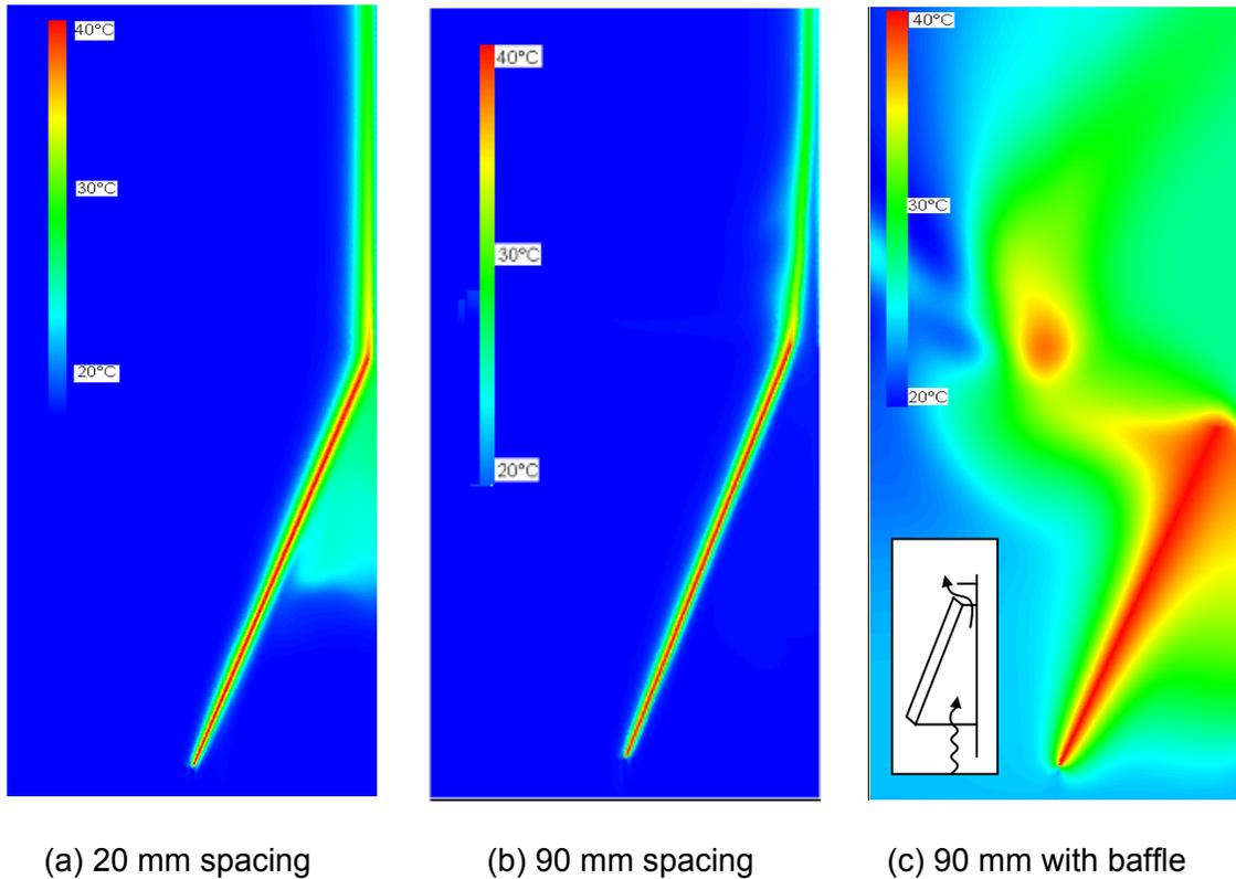
Fig. 9. Relative temperatures and flow field around the PV array for an assumed PV panel temperature of 40°C, an ambient temperature of 20°C, and a 24°C wall temperature above the array. Results are shown for cases: (a) panel to wall distance = 20 mm; (b) panel to wall distance = 90 mm and; (c) 90 mm gap with deflector baffle located 90 mm above the array.
