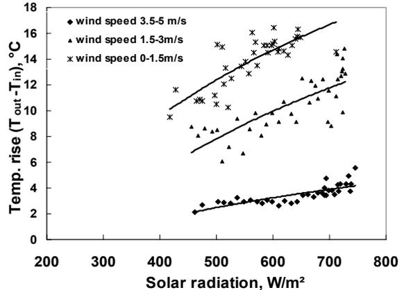
Fig. 8. Air temperature rise,  $(T_{out} - T_{in})$ , as a function of solar radiation and wind speed.
