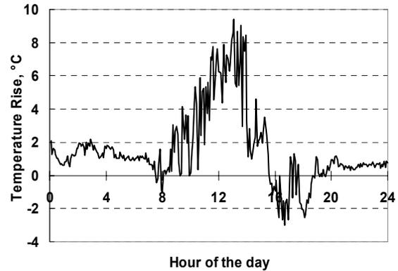
Fig. 7. Increase in air temperature above the ambient at a location 0.3 above PV panel (28/05/2002).
