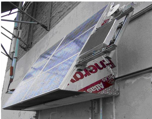
Fig. 3. Test section showing the insulation of the sides used to mimic a continuous array.
