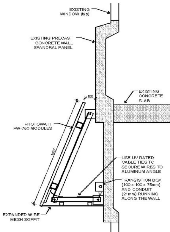
Fig. 10. Revised specification for attachment of the PV modules to the building wall [2].
