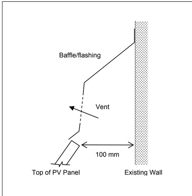
Fig. 12. Configuration of the baffle/flashing used above the PV arrays, (side view, not to scale).
