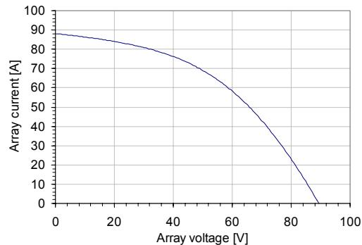
Figure 4 IV-curve of the parallel-only array.
