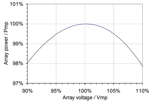
Figure 6 Power vs. voltage, close-up, parallel-only array.
