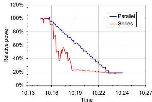
Figure 11 Total output of 5 modules during the first shading sequence
