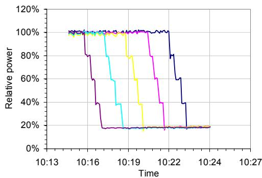
Figure 10 First shading sequence as measured on the five parallel modules
