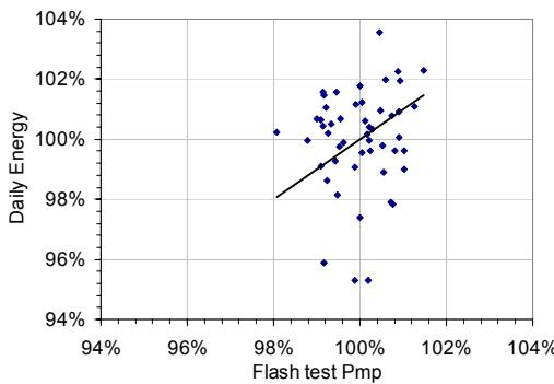
Figure 1 Energy output for a sunny day compared to factory flash test rating for 50 modules.
