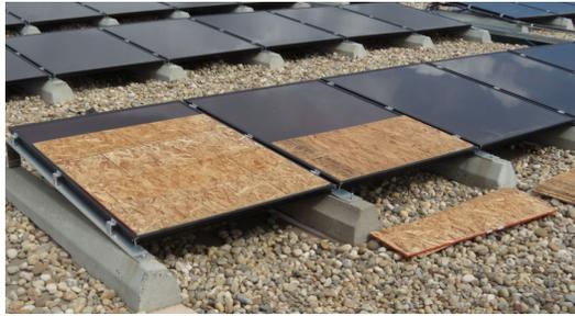
**Figure 9** Shade is created by wood panels in 20% increments
