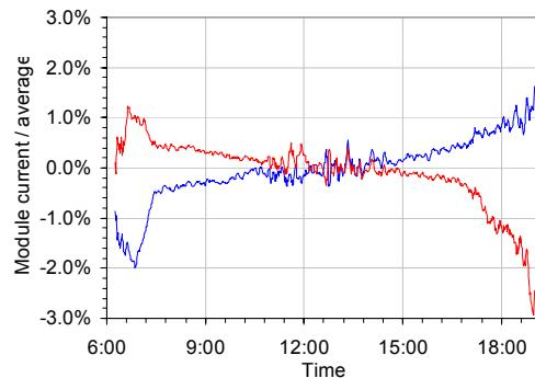
Figure 3 Relative output of two modules with opposing side-to-side tilt: red tilted East; blue tilted West.
