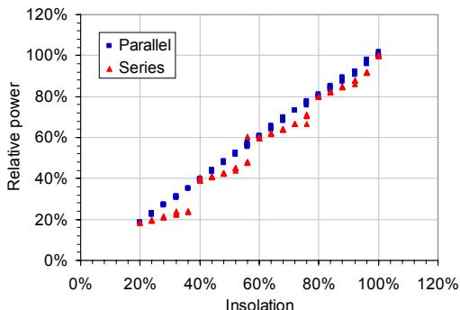
Figure 15 Output power as a function of insolation
