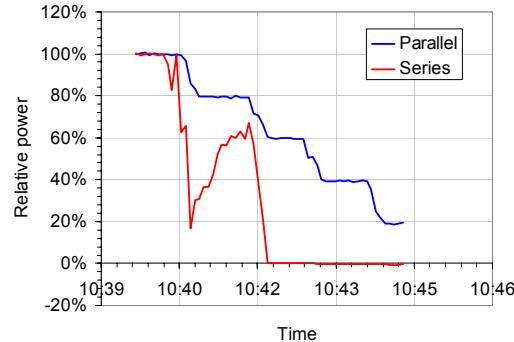
Figure 16 Total output of 5 modules with one, two, three and four modules covered completely
