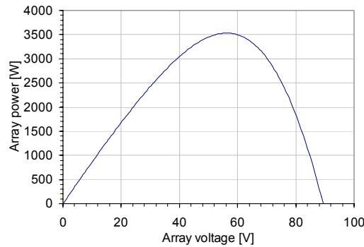
Figure 5 Power vs. voltage, parallel-only array.
