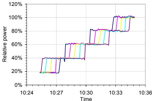
Figure 13 Second shading sequence as measured on the five parallel modules
