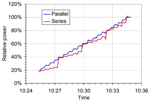
Figure 14 Total output of 5 modules during the second shading sequence
