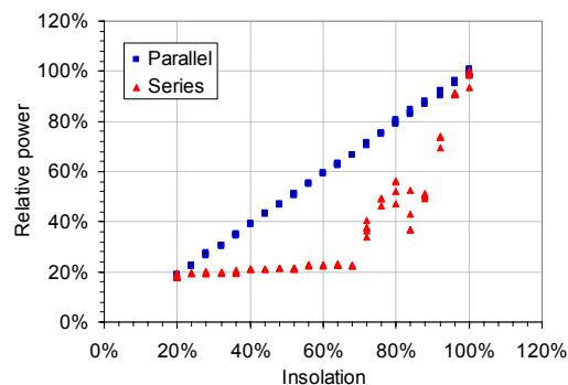
Figure 12 Output power as a function of insolation
