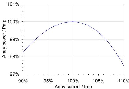
Figure 7 Power vs. current, close-up, parallel-only array
