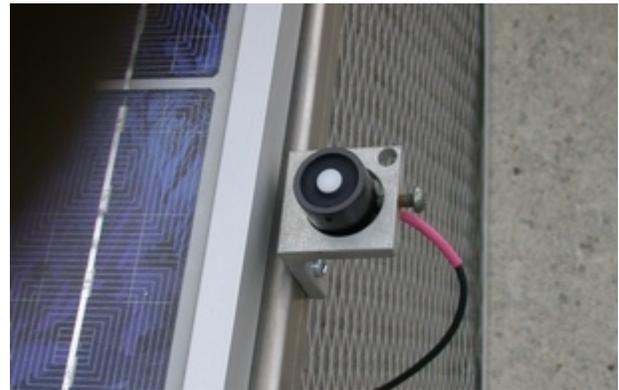
Fig. 2: Pyranometer mounting location.
