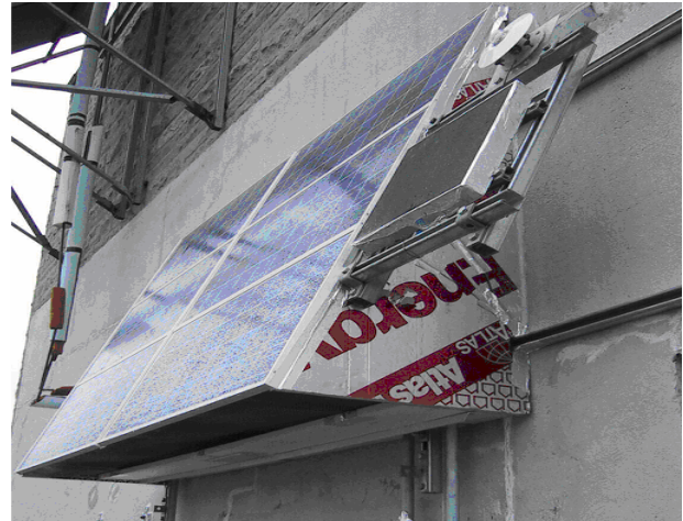
Fig. 3. Side view of test section showing the insulation of the sides to mimic a continuous array.
